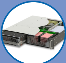
Redundant Power Supplies Single or Dual RAID Controllers
