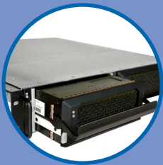
Enclosed & Electrically Isolated Drive Magazines
